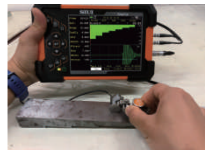
With PES-02D for encoded B-Scan
